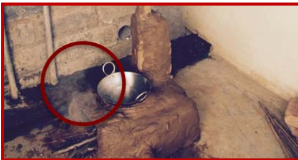
Figure 12. Smoke leaving from front opening during testing; side pipe covered. (Zhang, 2016)
