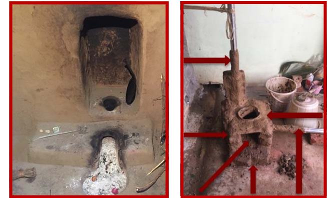
Figure 11. Comparison of traditional stove in Nehri Village to second prototype. Arrows note the changes made, which include a box-shaped stove, a closeable front opening, a top and side pipe, a closed stovetop, and a baseplate. (Zhang, 2016)
